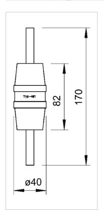
Closed, lightning current carrying spark gap for separation of electrically conductive plant components.
